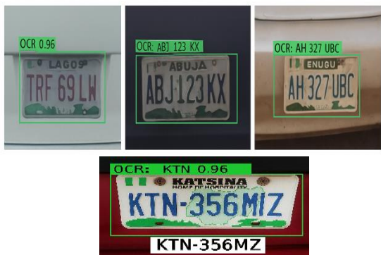
Figure 4: Detection of Nigerian plate using Faster R-CNN + OCR
